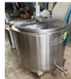
Bulk Milk Cooler 500L
